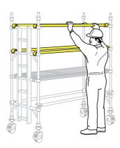
Fit 2 diagonal braces in opposing directions between the 1st and 3rd rungs. Ensure the frames are vertical and I evel by checking with a spirit I evel and setting the adjusta ble legs as necessary. Fit stabilisers (see notes on page 30). Fit the next pair of end frames and check the frame interlock clips are en gaged.
